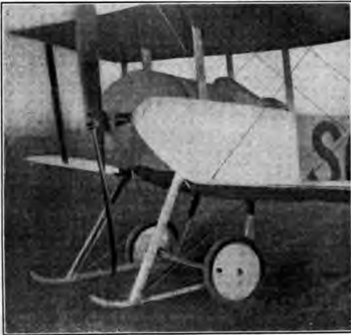
FIG. 6. SOPWITH CHASSIS, SHOWING COMBINATION OF TWO WHEELS WITH SHORT SKIDS
